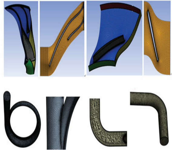
Fig. 27 Grid system of two-stage compressor
