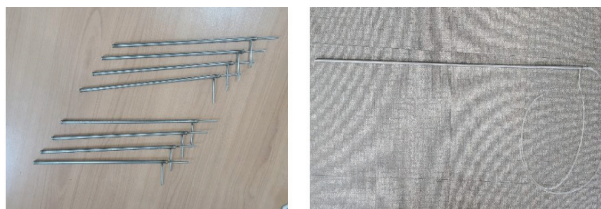
Fig. 6 Pitot tube for motor
