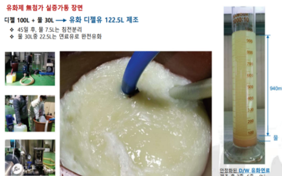
Fig. 10 Fuel Oil Test Scene with Nano Emulsion
