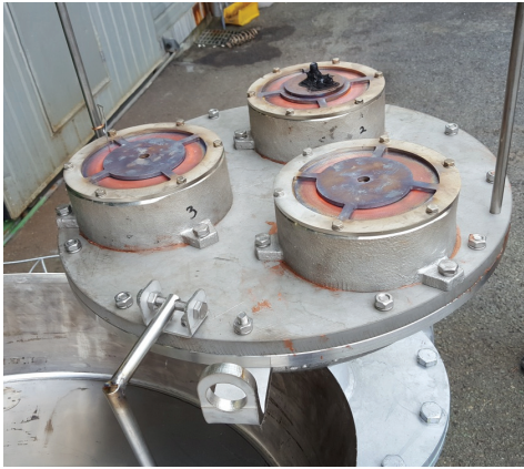
Fig. 10 Endurance burning test for prototype marine end-line flame arrester
