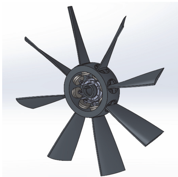
Fig. 2 3D Modeling of Scaled of Variable pitch Impeller
